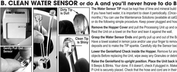
The Water Sensor TIP must be kept free of lime and mineral build up. If you have hard water, it is important to clean it periodically. (Once every 3 months.) You can use the Maintenance Solutions (available at catGenie.com) or do the following simple procedure. Keep power plugged and hoses in place.
