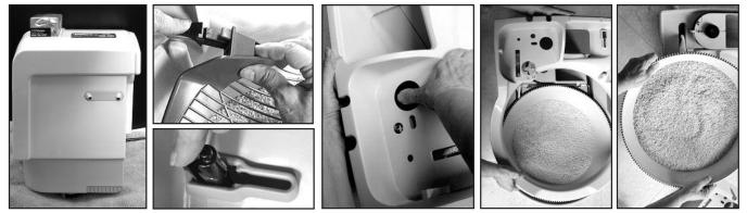
**To take apart your CatGenie**, move the CatGenie away from the wall. Keep the DrainHose in the toilet or drainpipe. Take off the Hopper Cover. Remove the Processing Unit and place it upright on a towel on the floor. Lean the Unit securely against the wall. Unclip
